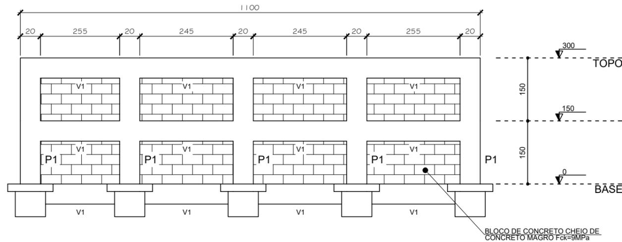
DETALHE TÍPICO DE MURO DE ARRIMO - 2,00m ATÉ 3,50m
